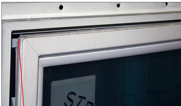
Window without Corner Drive: Noticeable separation in top corner of window at DP75
