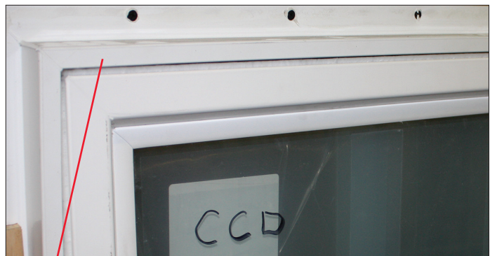
Same window with Roto LB11 Corner Drive: Top corner of window show minimal deflection at DP85
