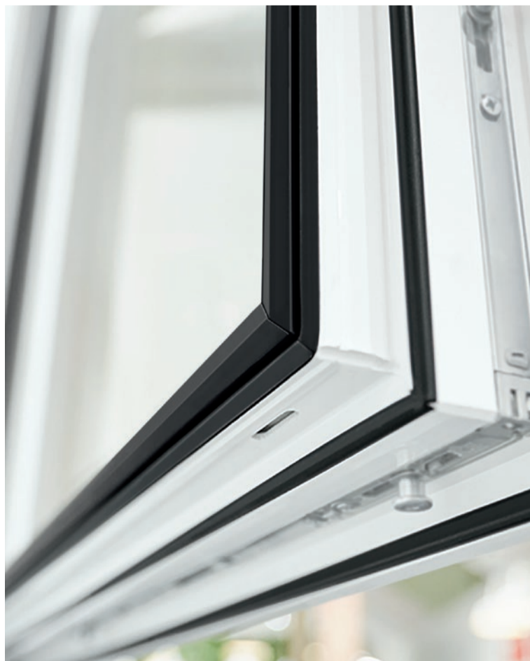
Adhesive tape, which is attached at the factory, secures the SP 7447 K sealing profile to the glass in the form of a stop gasket and glazing gasket. A large hollow chamber enables high tolerance compensation. Image: Gealan Fenster-Systeme GmbH
