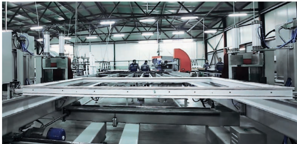
The Belarusian Market leader of PVC and aluminium building elements based in Mogilev has a production capacity of around 1,500 window units per day. The production volume can be doubled whenever necessary. Images: Avansum
