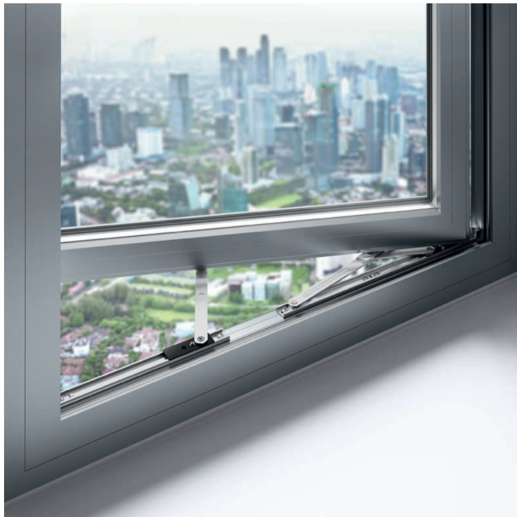
A concealed lock improves the sealing, especially with large window formats, and reduces deformation of large Top-Hung sashes caused by wind loads. Several versions are available for different profiling types.
