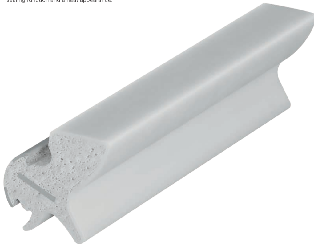
Perfect in the corners: Master Corner – the TPE profile with patented new technology for closing characteristics that are the same all around the circumference, with optimal sealing function and a neat appearance.
