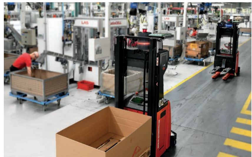
Driverless transport systems replenish semi-finished products for workstations in production.
