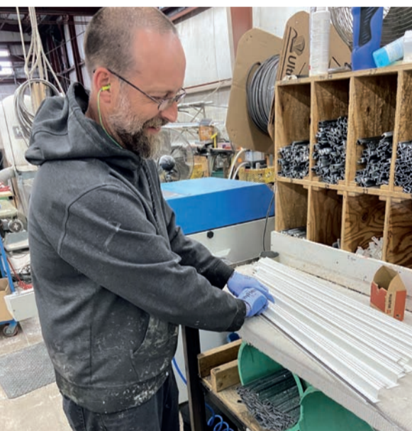
Jim Adams inserts Ultrafab weather seals into vinyl profiles.
