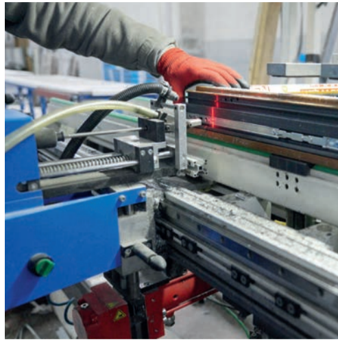
Screwdriving robots ensure optimum torque during hardware installation.
