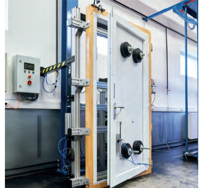
Durability test in accordance with DIN EN 1191 in the accredited test centre at the Kalsdorf ITC
