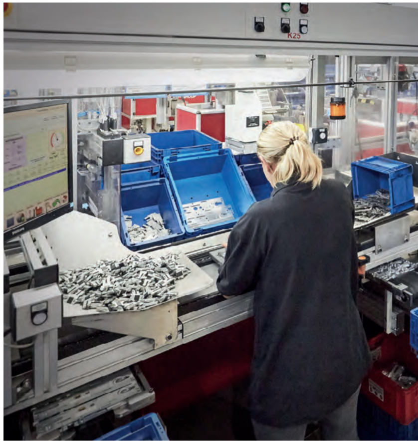
Around 80% of the Roto multipoint locks sold worldwide are produced in Kalsdorf. Identical parts and large series are manufactured in a semi-automatic process. As ever, the smallest series are produced the most efficient way – manually.
