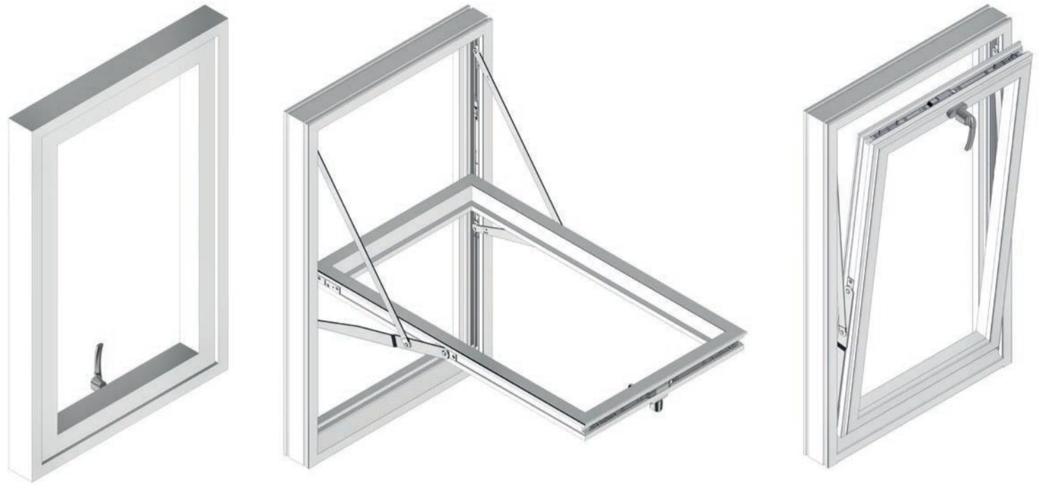
Turn the handle and open the element – push the sash outwards and turn it fully to clean the outer side.
