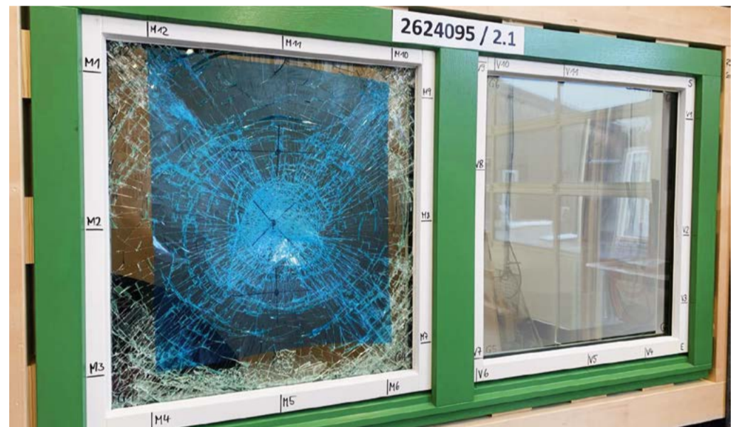
"Security" product world: test passed! Grünbeck produces single- and double-sashed timber windows up to resistance class RC 3 with the Roto NX Tilt&Turn hardware.
